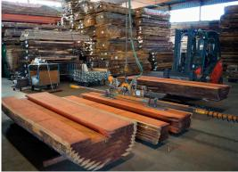
left: Table top is lifted onto the milling table using a vacuum crane above: Measuring padouk
