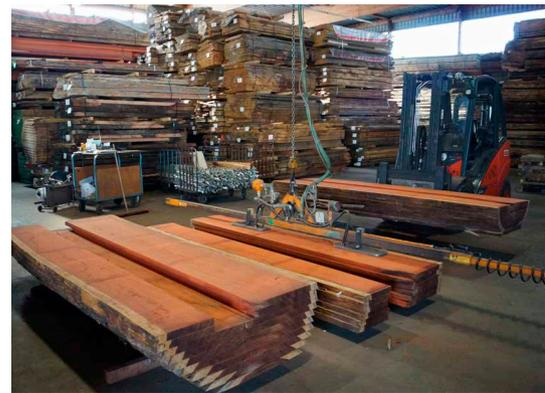
left: Table top is lifted onto the milling table using a vacuum crane
